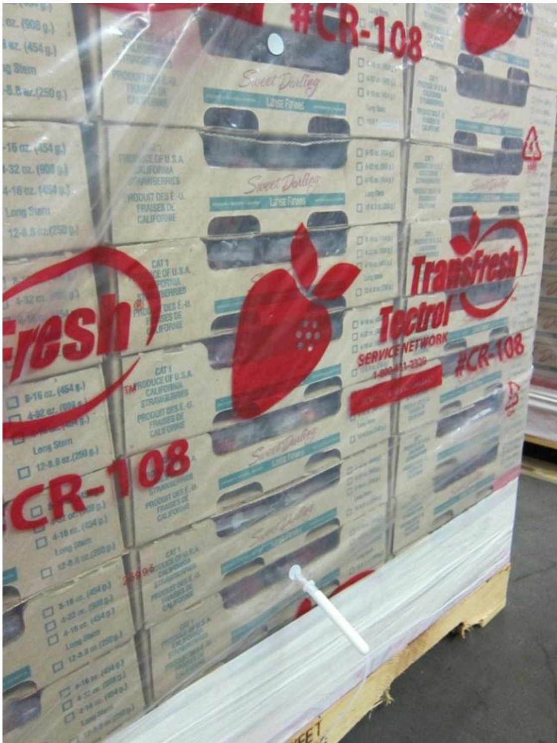
Fig. 3. Gas sampling from pallet treated with the Tectrol® system. Self-sticky resealable septa are visible at levels 3 and 9 on the pallet
