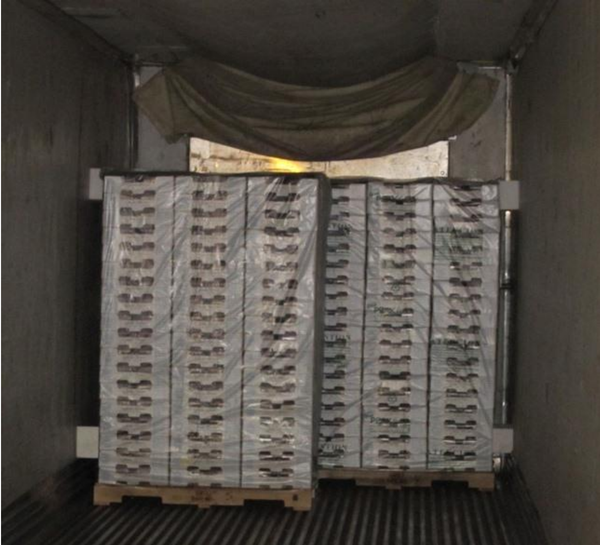
Fig.4. Pallets of strawberries placed in a pre-cooled trailer. The pallets have been overwrapped with PEAKfresh® strawberry pallet bags. Note that the bags are not sealed at the bottom and are open to airflow
